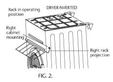
Rotate the door outlet grill so that the air exhaust blows upwards and through the rack.
